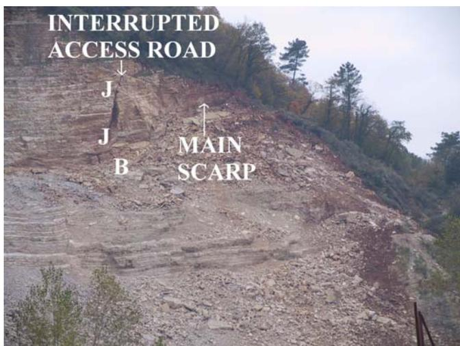
Fig. 3 Picture taken on 22<sup>nd</sup> November 2004 of the collapsed zone after the failure: JJ sub-vertical joint, B Block
