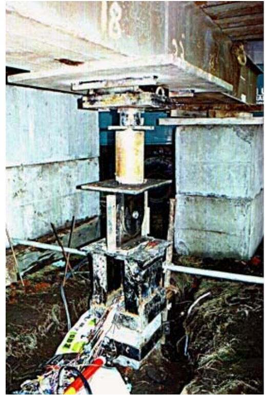
Fig. 4: Test setup at pile AL1
