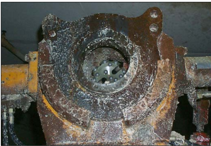
Photograph H – Downhole percussion hammer
