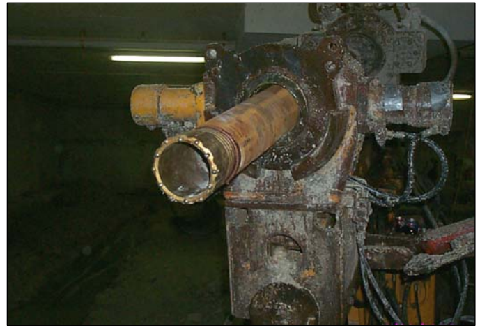
Photograph I – Casing used during drilling operations
