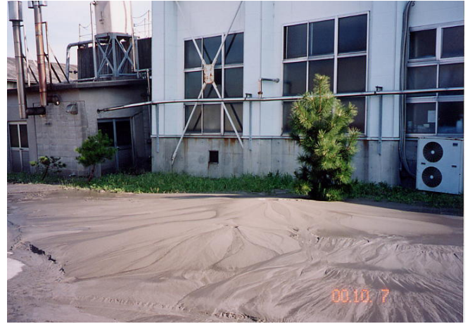
Photo 3. A big sand boil at an industry in Takenouchi industrial park
