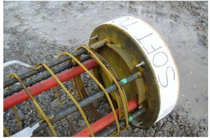
Figure 8 Soft pile toe used to eliminate base resistance in load tests on rock socket piles (See Paper 2.08)
