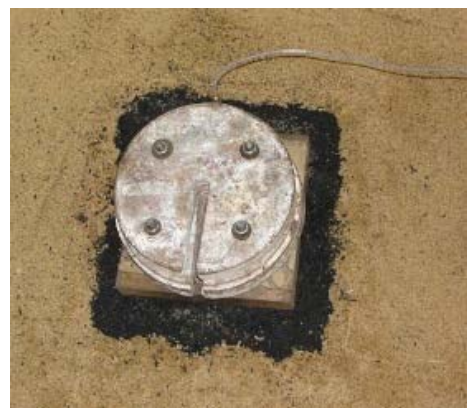
Figure 6. Model footing resting on shredded rubber and sand mixture.
