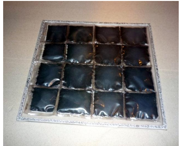
Figure 6-b. Polycarbonate small-scale structure model composed of a hollow slab and small bags of lead powder representing the load.
