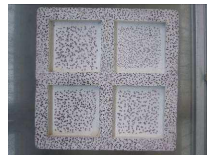
Figure 7. Silicon small-scale structure model composed of a hollow slab
