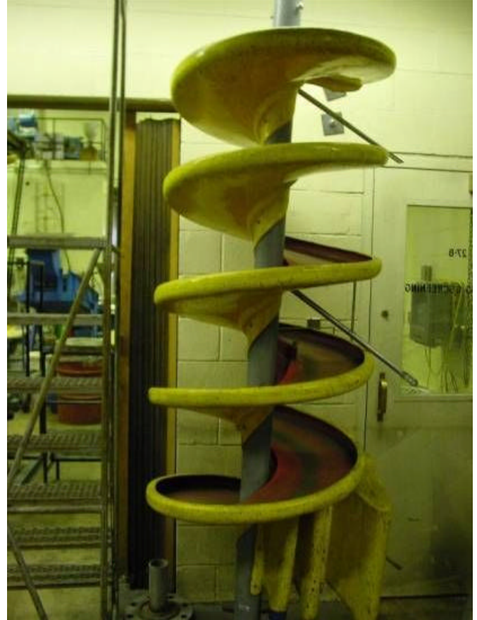
Fig. 3 – Five-Turn Spiral Concentrator
