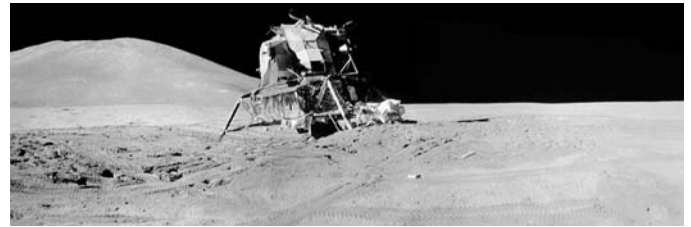
Fig. 2. Apollo 15 LM tilted backwards 11 degrees into a shallow crater.
