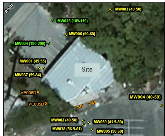
Fig.1. Site layout and location of monitoring wells.
