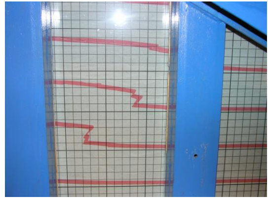
Figure 2b. Experiment E5/0,2: Detailed view of the deformed and failed area marked in Fig. 2a with a zone of a main system of the slip surface after rotation about the top (toe movement of u=+154.74 mm).
