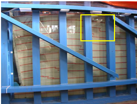
Fig. 3a. Experiment E6/0,2: View on the deformed and failed front section of the mass behind the moved front wall after rotation about the top and toe movement of u=+156.25 mm. A position of the front wall is very obvious on the left.
