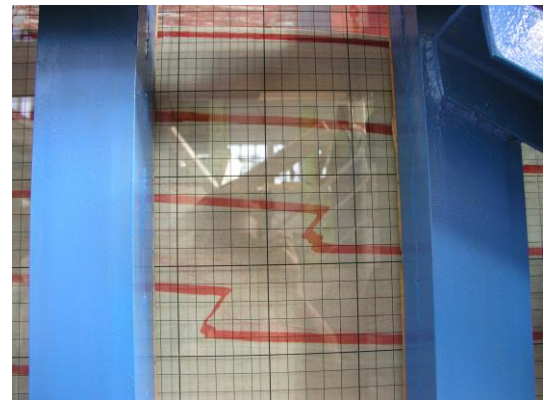
Figure 3b. Experiment E6/0,2: Detailed view of the deformed and failed area marked in Fig. 3a with a zone of a main system of the slip surface after rotation about the top (toe movement of u=+156.25 mm).
