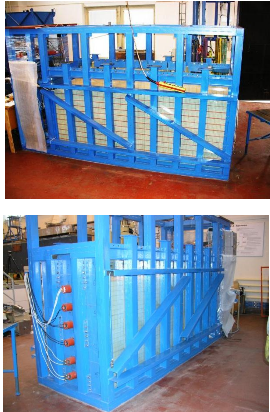
Fig. 1. Experimental equipment with transparent glass sides before experiment E5/0,2 with non-cohesive sandy sample into: a) (above) Lateral view at right equipment side. The moved front wall is left. b) (below) Lateral and back view at left equipment side. Front moved wall is right and back solid wall with one three-component and five bi-component pressure sensors is left.
