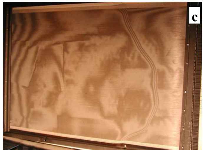
Figs. 2a,b,c. The final form of the ideal non-cohesive sandy mass after rotation about the top of the front equipment wall (in Figs. 2a, c left, in Fig. 2b before, down) and the toe movement of 159 mm:
