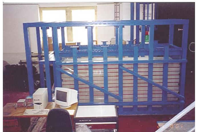
Fig. 1. General lateral view at the experimental equipment with sample of the ideal (dry) non-cohesive sand inside before the long-term experiment E3/2 (29 th Aug. 2001). The moved front wall is left.
