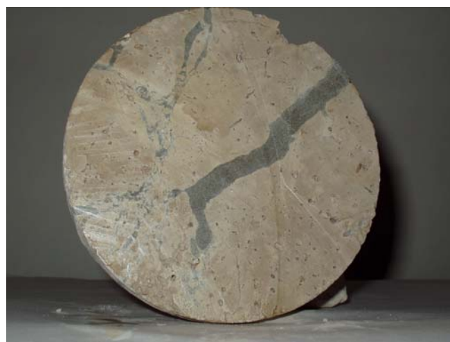
Fig. 2. Horizontal shear of the cement treated specimen
