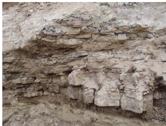
Fig. 1. Layer-flaggy structure of rocks with clear tracing of cement treatment
