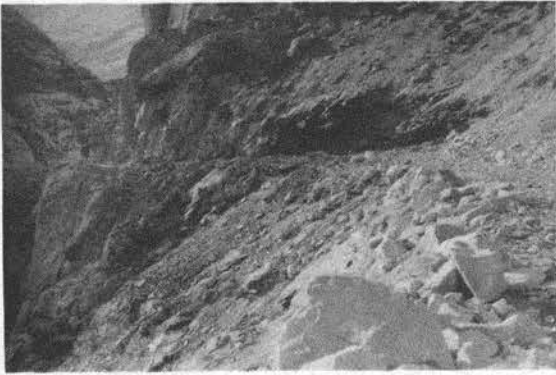
Fig. 18. Catastrophic failure of slopes along India-Tibet road in weathered and jointed granitic gneisses.
