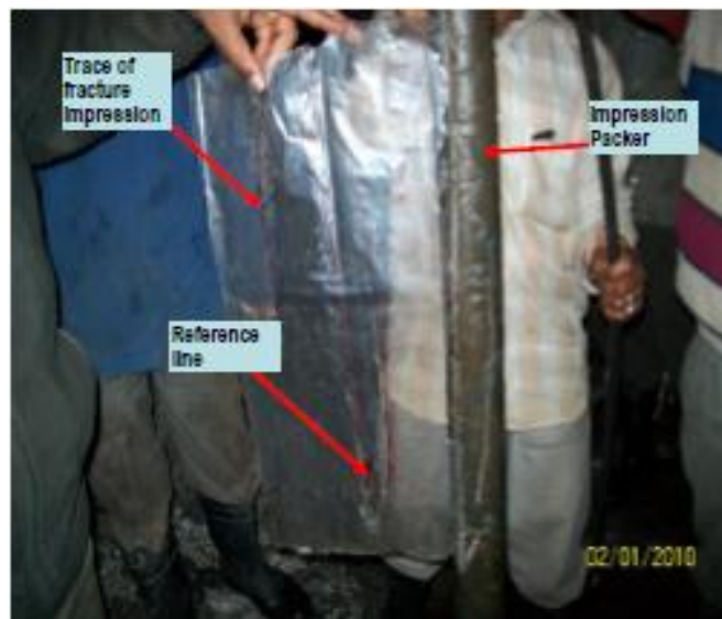
Fig. 7 Impression packer to know the fracture orientation Data acquisition system used during the test
