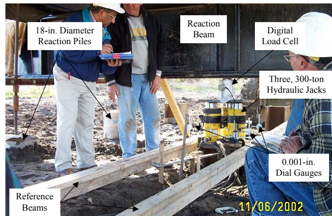
Fig. 3. General View of the Compression Test Apparatus and Set-Up (note that one additional dial gauge measuring pile head deflection and the tell-tale dial gauge are not visible in this photograph).
