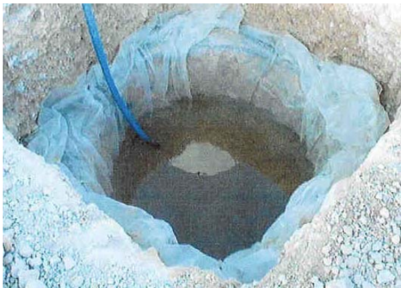
Fig. 10. Some views of large in-site density test
