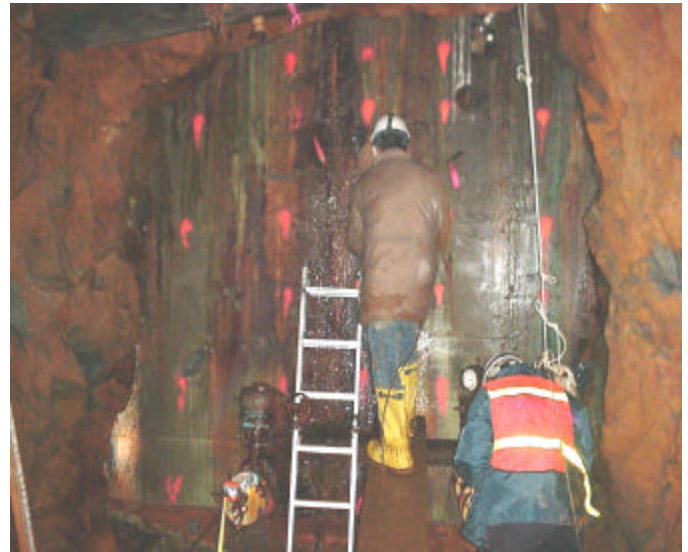
Photo 2. Seal on November 1, 2000. Red paint marks are impact points for nondestructive testing.
