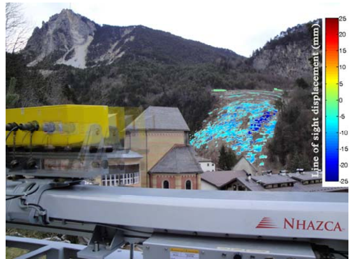
Fig. 6. Perspective view of the TInSAR interferometer IBIS-L and slope overlaid by the displacement map.
