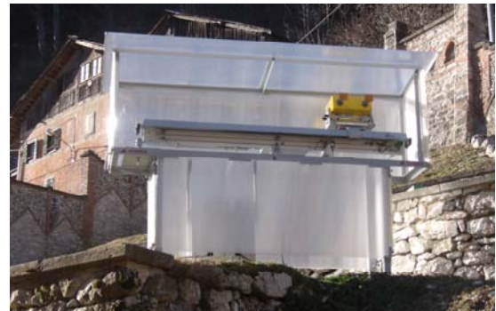
Fig. 1. Picture of the TInSAR system IBIS-L by IDS S.p.A. installed on a QUIB basement by NHAZCA S.r.l..
