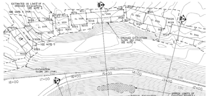
Fig. 19. Dredging Plan, West Dam.
