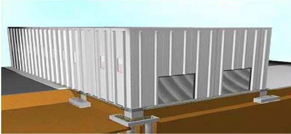
Figure 48. Section view of an existing industrial building in the examined area, with pile foundations.
