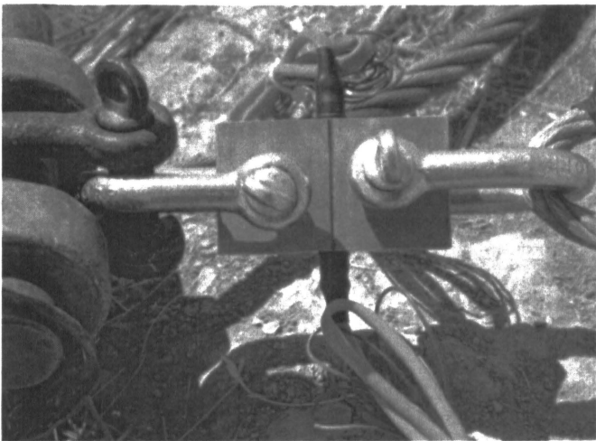
Fig. 6. Explosive tie allowing a sudden tension release
