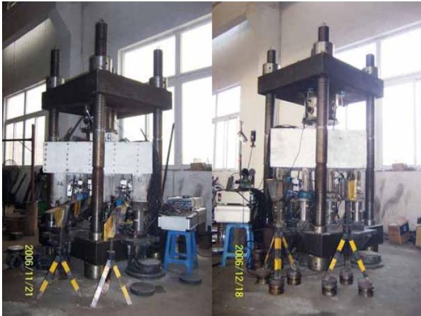
Fig.13. Testing setup (9-pile and 16-pile)
