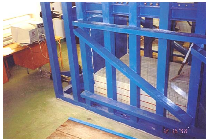
Fig. 10. Experimental stand with transparent lateral sides. The retaining wall is the blue plane inside the structure on the left. Two red sensors can be seen placed in the retaining wall through the front side. The other one above is not in place
