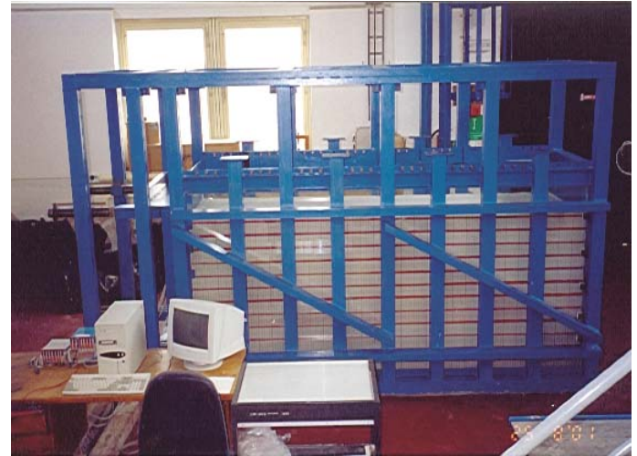
Fig. 12. Lateral view at the experimental stand and the sample of granular mass into. The arbitrary moved front wall is left. State before the experiment E3/2 (passive rotation about the top) on 29 th Aug. 2001.
