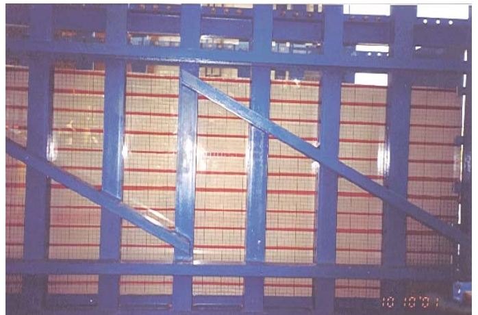
Fig. 13. Lateral view at the experimental stand and the sample of granular mass into after rotation of the toe of 17.5 mm about the top. State during the experiment E3/2 (passive rotation about the top) on 10 th Oct. 2001 before the movement stop for the time (in)stability experiment.
