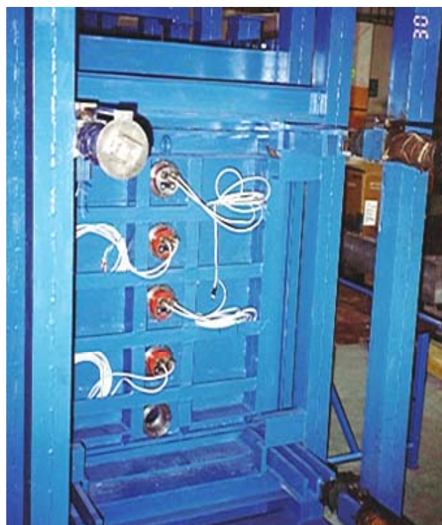
Fig. 11. Front space of the retaining wall with 4 bicomponent tensors. The lower is not in place.
