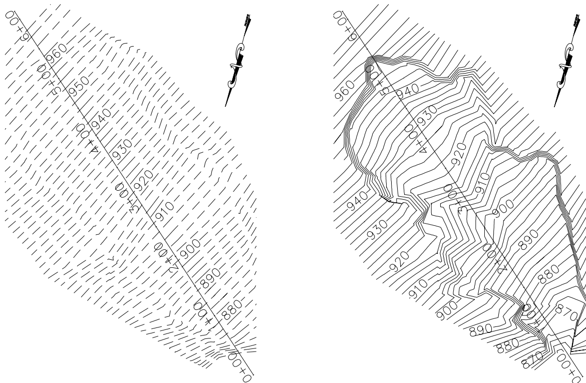
Fig. 6. Topography of rupture zone prior to the slide (left). Topography of rupture zone after the slide (right).
