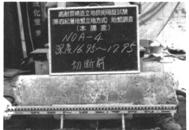
Fig.6 Frozen gravel sample from a core-barrel
