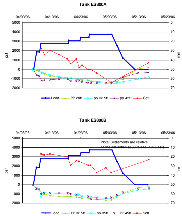
Fig. 22. Tank ES800s Piezometer readings, loading history and inferred maximum settlements during hydrotest
