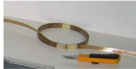
Fig.3. Coil of the optical fiber sensing tape
