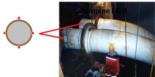
Fig. 4. Location of strain gauges
