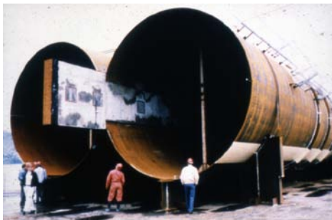
Fig. 1. Lower end of test structure. Instruments for measuring soil friction, pore water pressure and earth pressure on the concrete panel can be seen.
