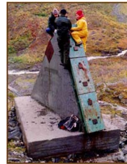
Fig. 3. Test structure with 3 load plates to measure impact forces during an avalanche (1982)
