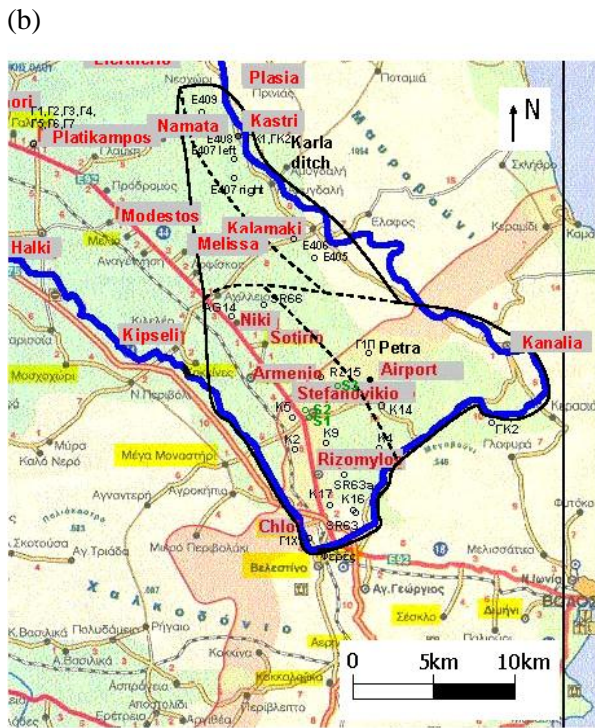
Fig. 2. (a) Eastern Thessaly accretional basin and (b) Karla region. S1 indicates the site under study. Notations ( \Gamma , E ) indicate geotechnical borings. All other notations ( K , ...) indicate piezometer positions.
