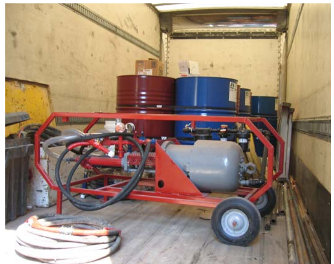
Fig. 8. Component “A” and “B” barrels and two-sided pump.
