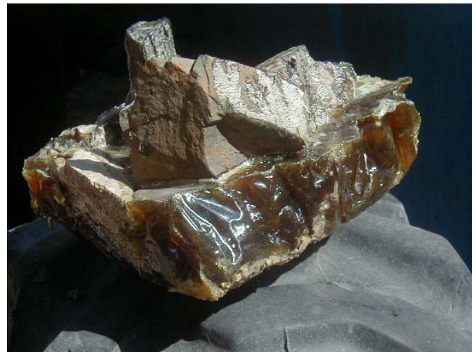
Fig. 1. Rock fragments permanently bonded within hardened polyurethane resin (PUR).
