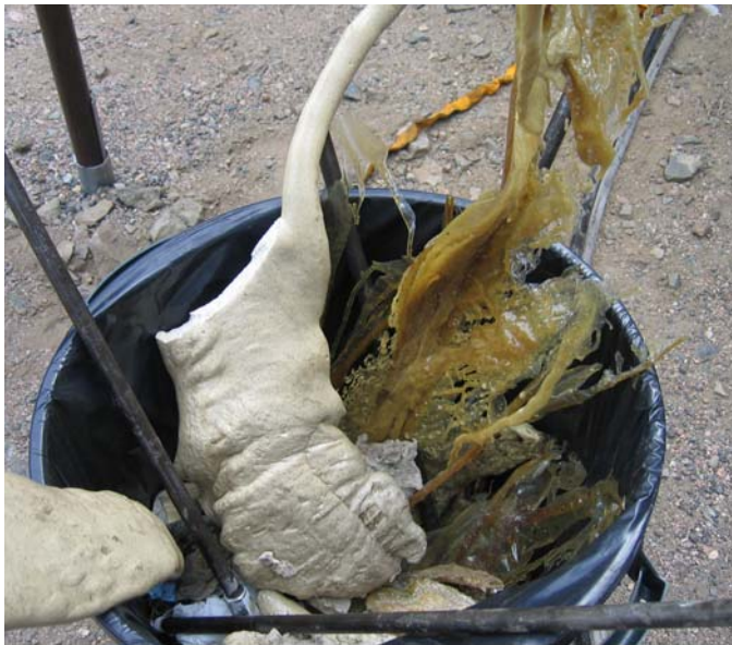
Fig. 4. Examples of non-foamed PUR (brown resin material) and foamed PUR resulting from contact with significant moisture (light tan material).
