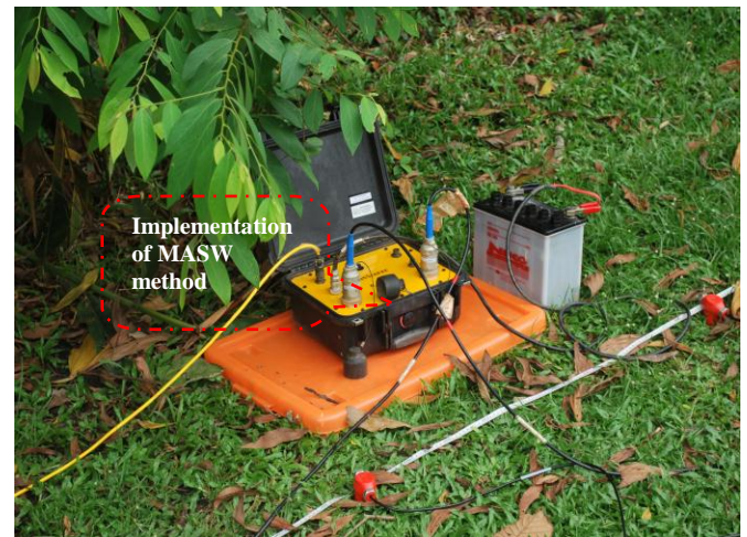
Fig.3. Seismic data acquisition at near of landslide occurrence
