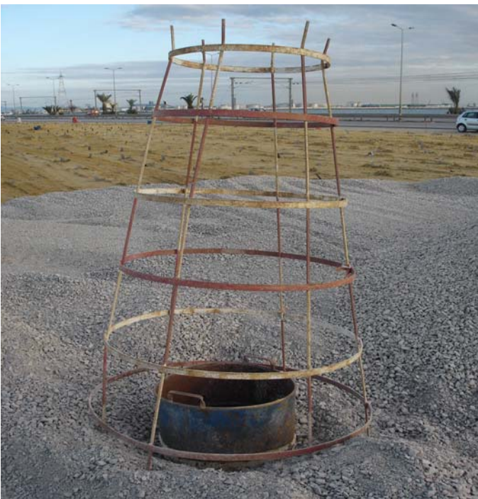
Fig. 16. Protected settlement recorder.
