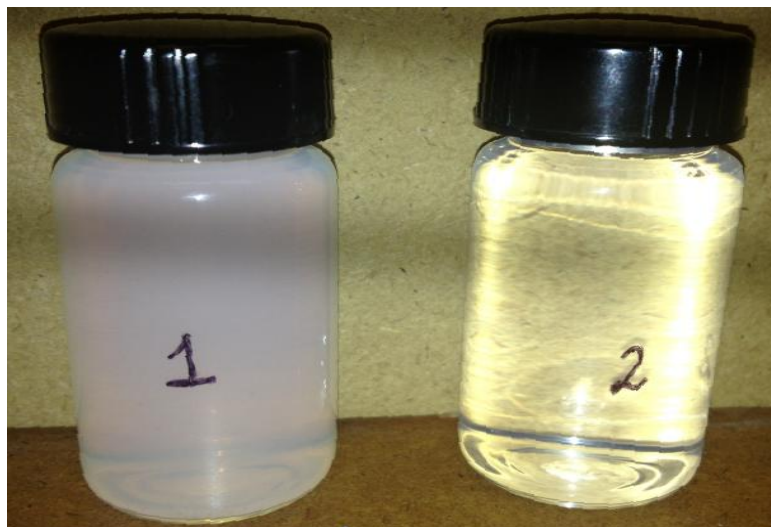
Figure 6. Vial 1: improperly water-reduced CUPs; Vial 2: properly water-reduced CUPs
