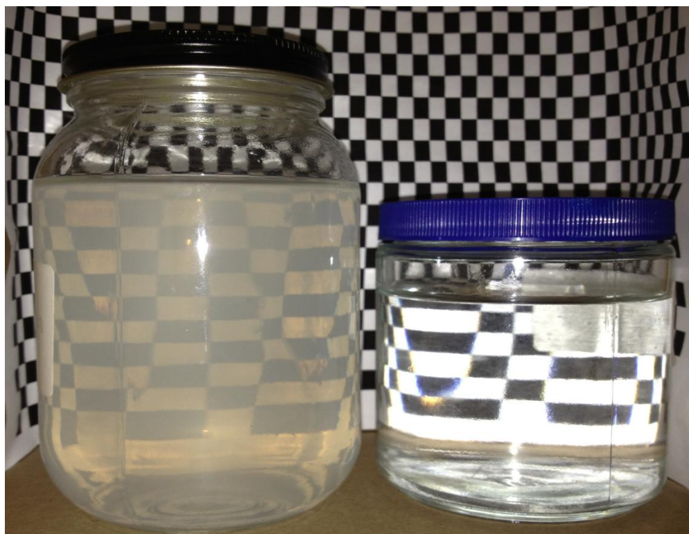
Figure 6. Jar 1: improperly water-reduced CUPs; Jar 2: properly water-reduced CUPs.
