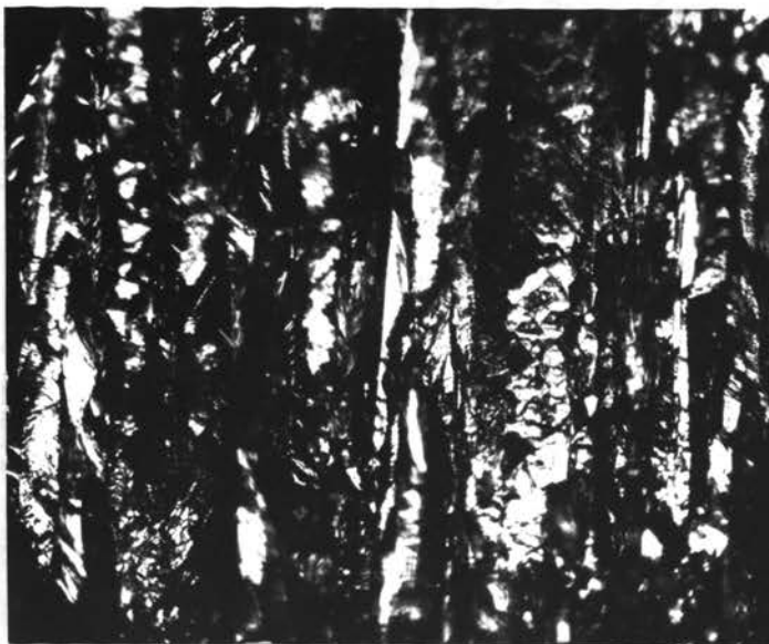
Figure 39. Columnar structure of electrolytic iron used for anodic dissolution. x 150.
