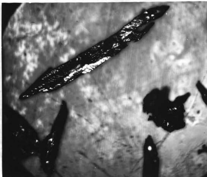
Figure 38. Particles formed due to anodic disintegration of electrolytic iron having a fiber-structure(see next Fig.) in 6 N H_2SO_4 . x 150.
