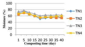
Figure 2: The variation in moisture by the composting times.
