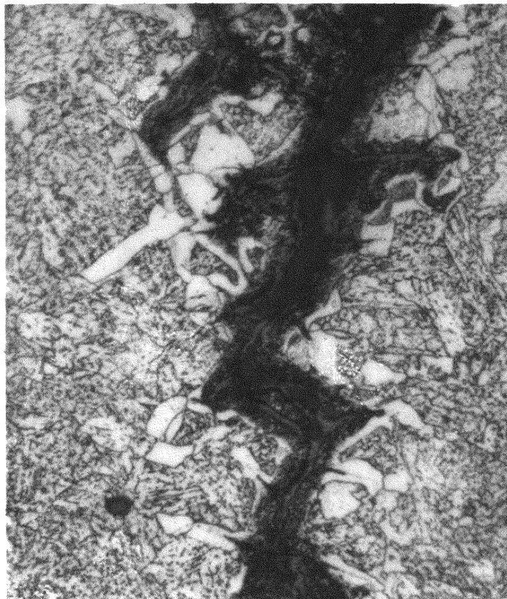
Figure 12. Photomicrograph of crack representa- tive of high \text{CO}_2 specimens, nital etch. 500X
