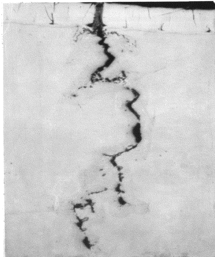
Figure 14. Crack propagation in the absence of pitting in Cr plated specimen. 50% CO 2 , unetched. 500X
