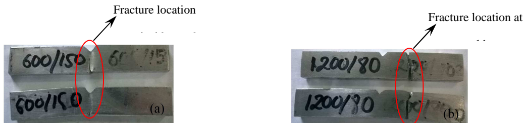
Figure 12. Fracture locations of weld regimes \omega/v = 4.0 rev/mm (a) and \omega/v = 15.0 rev/mm (b).
