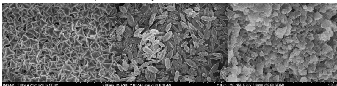
Figure 2. The SEM images of the MIL-53(Fe), MIL-88(Fe), MIL-100(Fe) materials.
