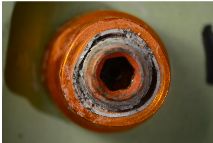
Figure 4.23. Post-Test Stress Corrosion Fastener 11 Collar
