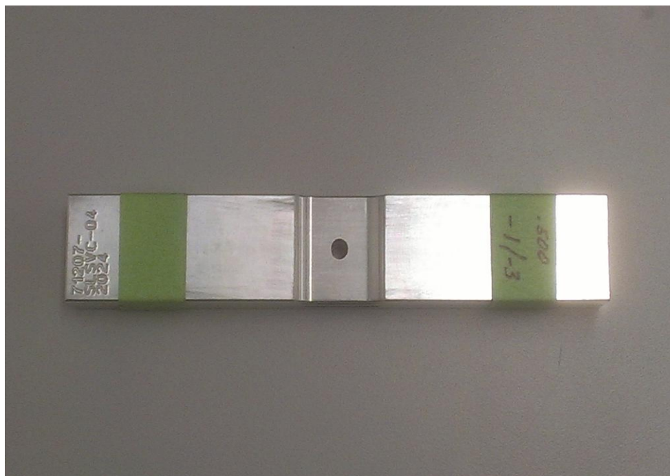
Figure B.2. Open Hole in Radius Test Specimen -2 Pre-Test Picture
