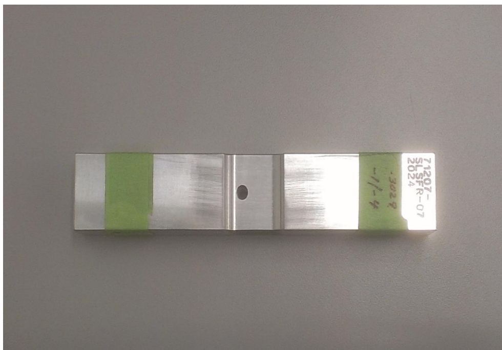
Figure B.4. Open Hole in Radius Test Specimen -4 Pre-Test Picture
