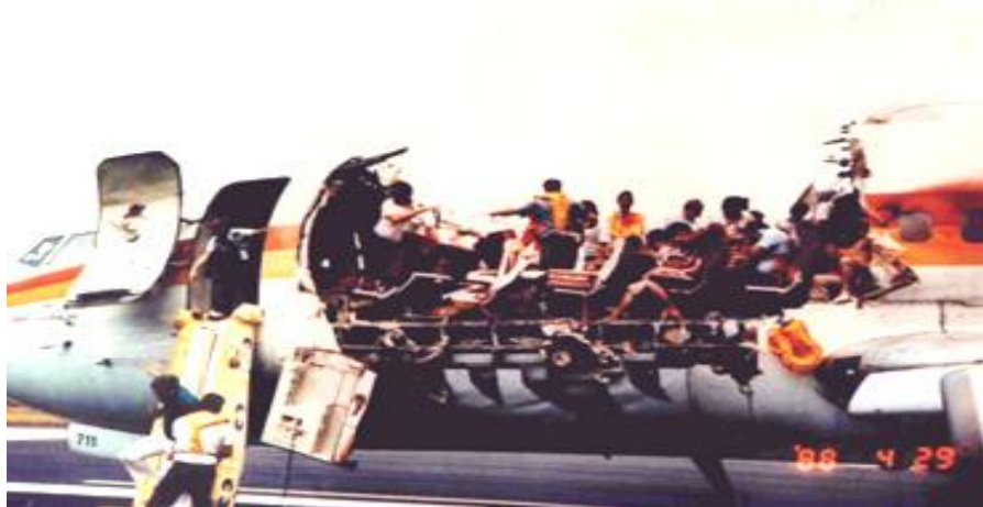
Figure 1.2. Aloha Airlines Flight 243 - Fatigue Failure Due to Corrosion [6]
