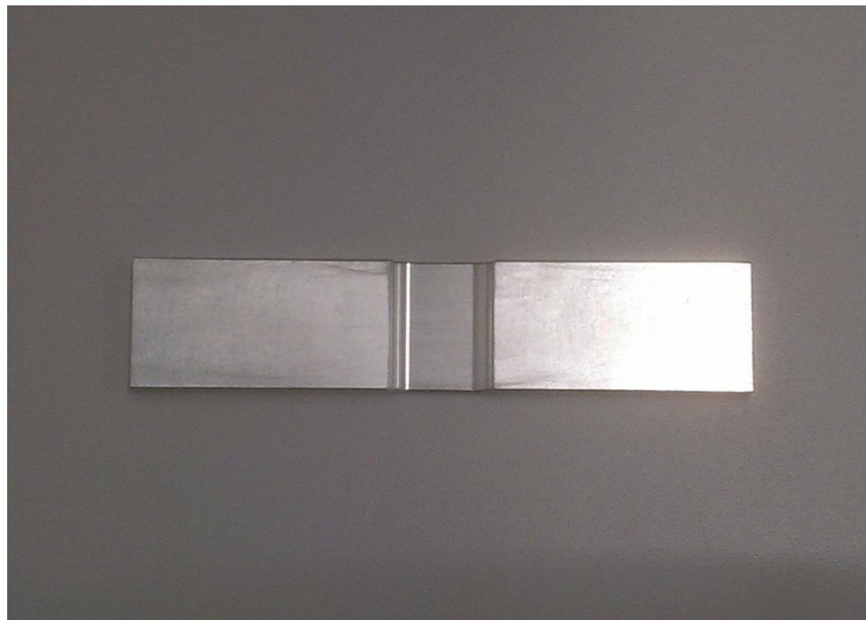
Figure B.1. Open Hole in Radius Test Specimen -1 Pre-Test Picture
