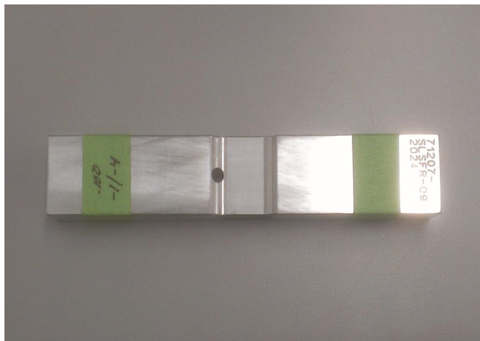
Figure B.6. Open Hole in Radius Test Specimen -6 Pre-Test Picture
