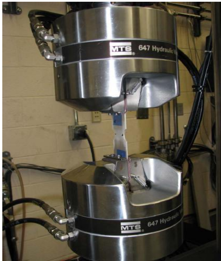
Figure 4.2. MTS 810 Material Testing System
