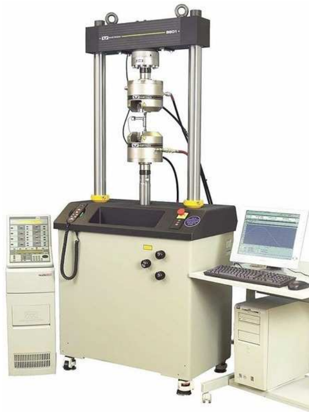
Figure 4. Servo-hydraulic axial fatigue tester (www.directindustry.com n.d.).
