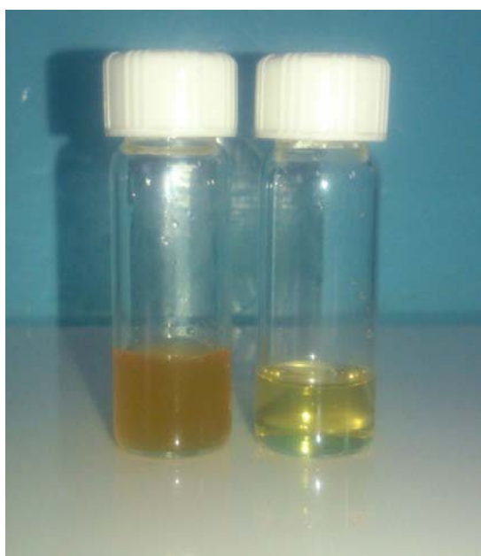
Figure 4. The change of OS solution stage with the change of pH: OS solution at pH > 10 (on the left); OS solution at pH < 4 .
