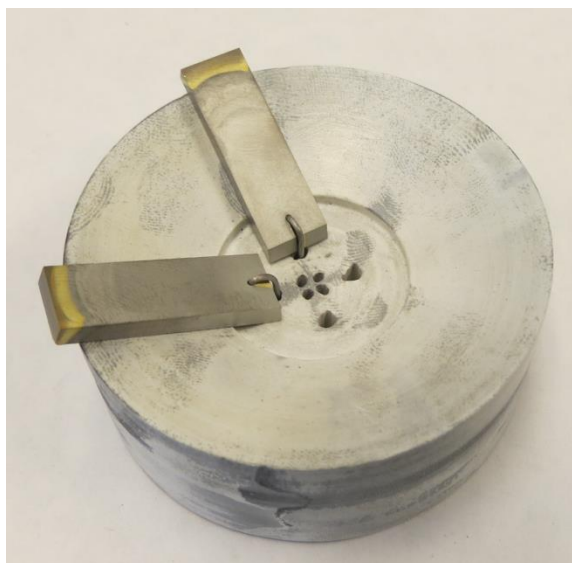
Fig. 26. Boron nitride setter with ZrB_2 contacting bars set in the conical depression. The bars can also be seen with tungsten wires inserted.
