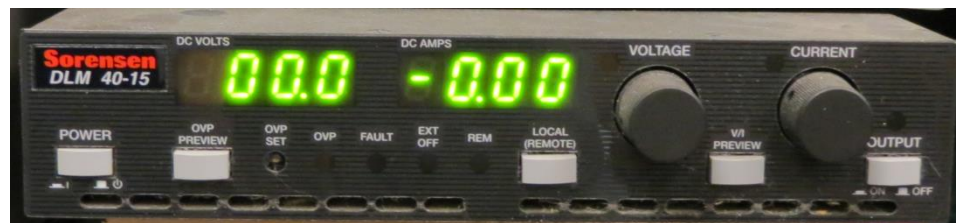
Fig. 7. Front interface of the DC power supply which displays the applied current and corresponding voltage; and allows for manual control.
