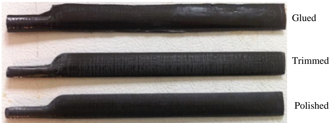
Fig. 3 Manufactured AS4/Cycom 5320 composite blades
