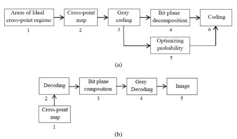
Figure 2. The scheme of 2-DICRIC with two processes - (a) Compression - (b) Decompression.
