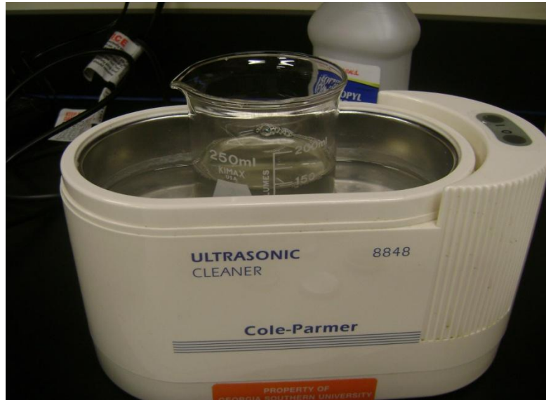
Figure 48: Ultrasonic bath of the disk with indirect method
