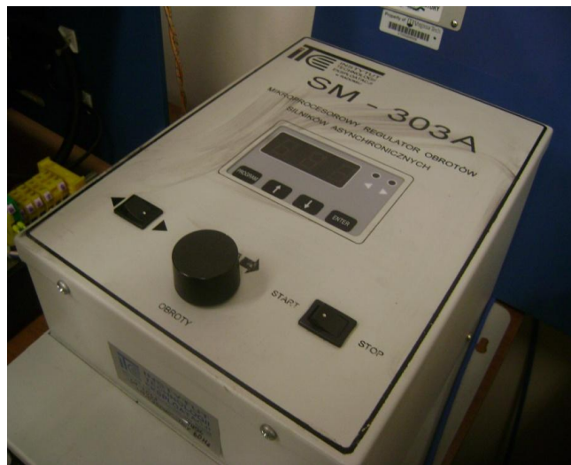
Figure 37: Motor speed controller
