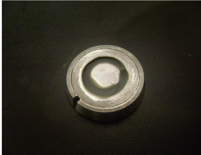
Figure 68: The left over oxidized oil after a test run with a typical SOB diluted EO
