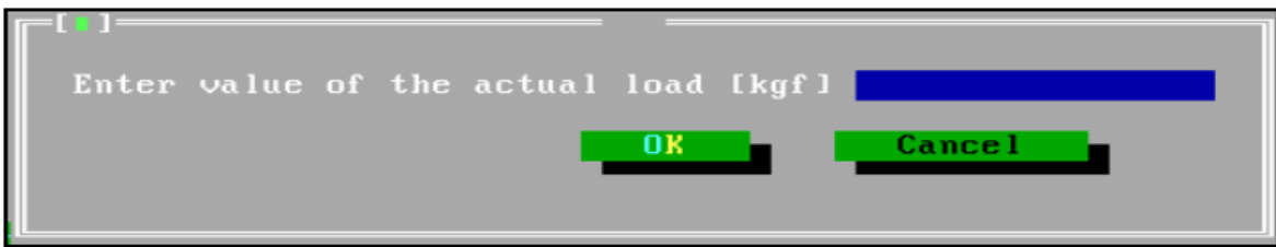
Figure 44: Dialog box of entering current load value for frictional force calibration with T-11 program. (Tribology, 1994)
