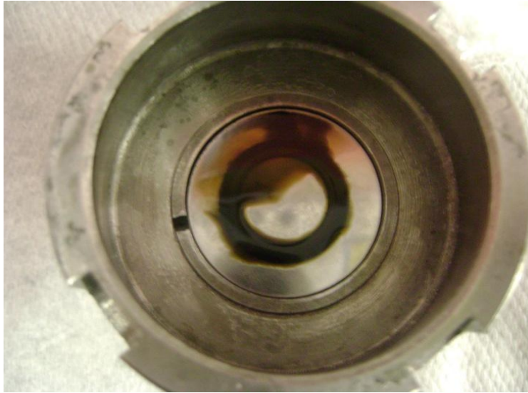
Figure 55: The left over oxidized oil after a test run with a typical COB diluted EO.
