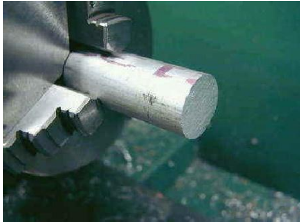
Figure C2: The chuck holding the round bar in the parting operation.
