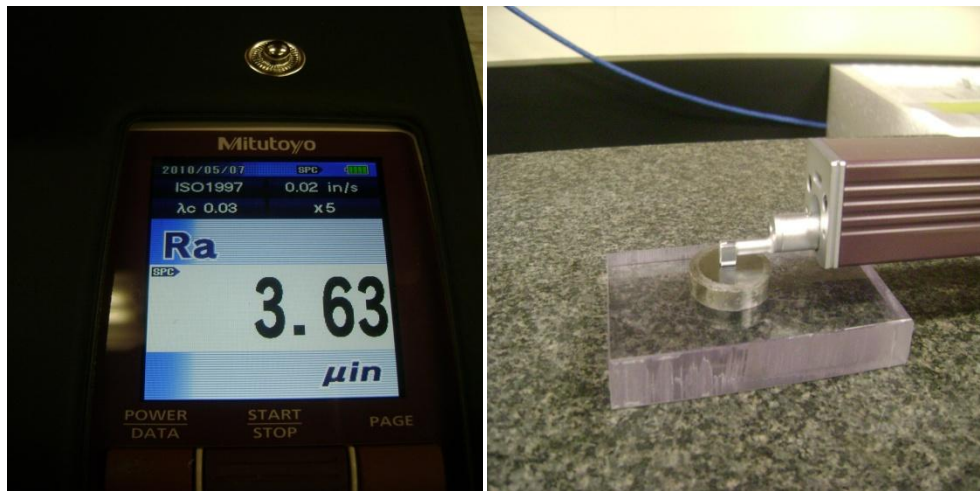
(a) Stylus movement along the surface
