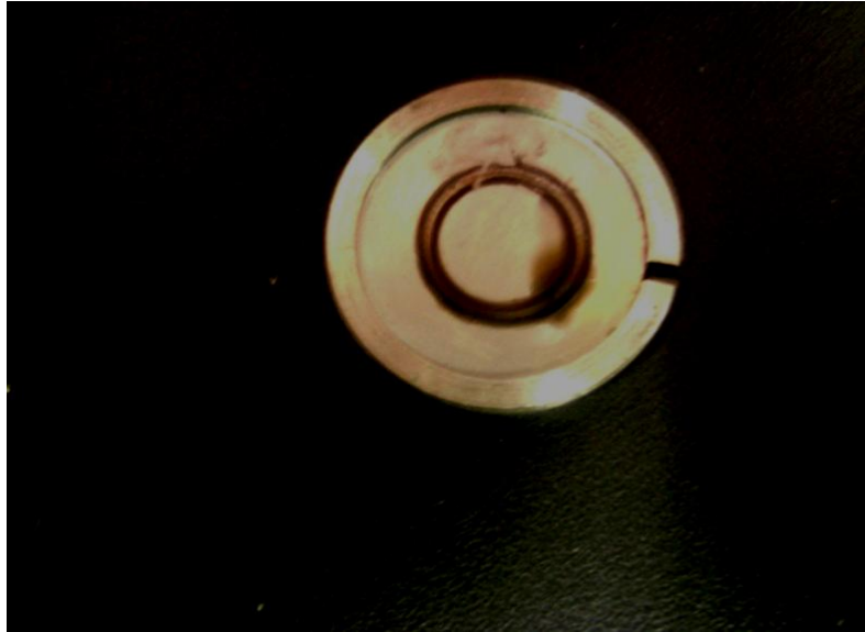
Figure 62: The left over oxidized oil after a test run with a typical POB diluted EO
