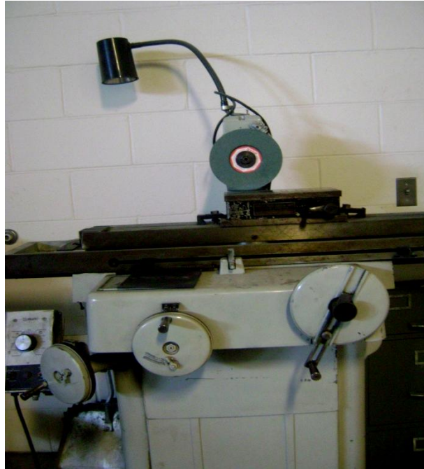
Figure C8: Surface grinder used for surface finish.
