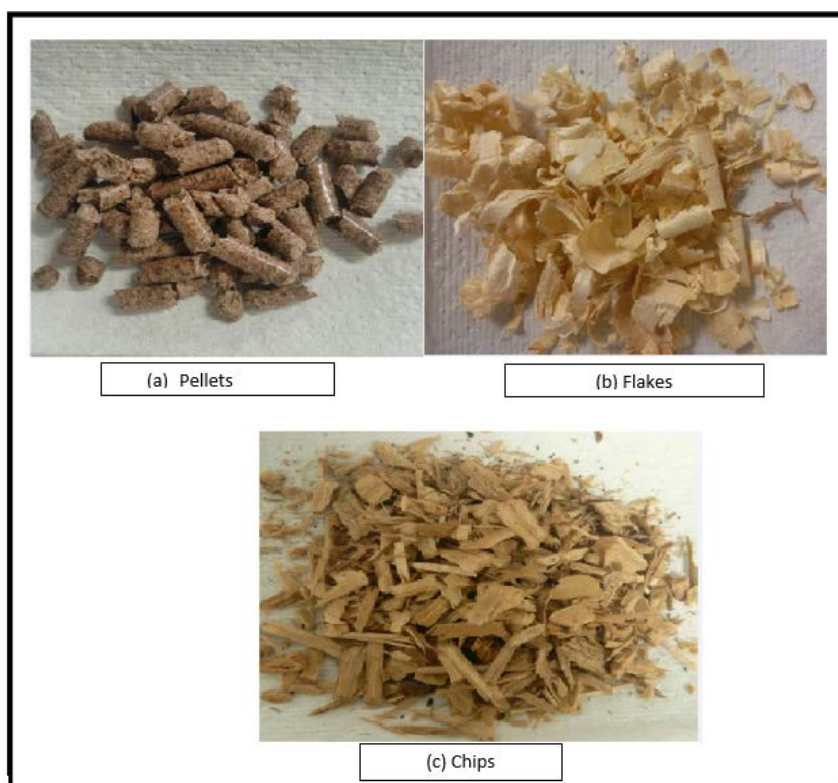
Figure 2.1. Different types of feed used in Missouri S&T energy center lab
