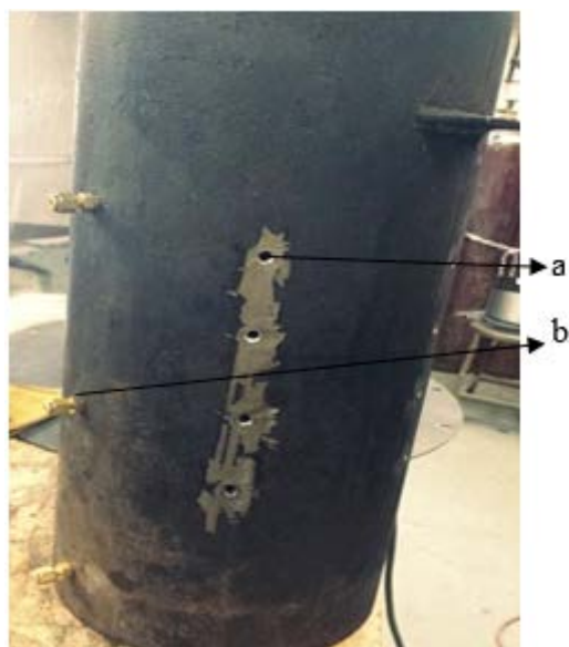
Figure 2.2. Reactor core with a) Air nozzles and b) Thermocouple openings
