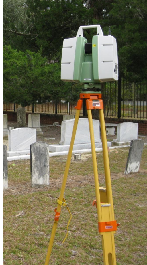
Figure 22: Leica C10 LiDAR Scanner
