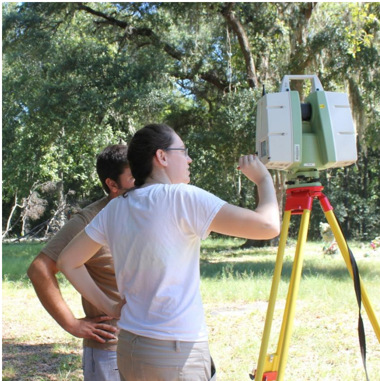
Figure 16: Leica C10 LiDAR Scanner
