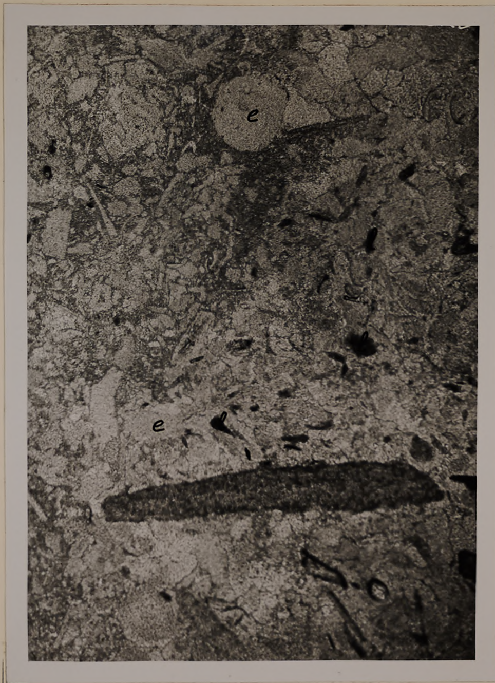
Plate XIV Photomicrograph of a representative thin section (CK 2 ) of the Cape Limestone from Cape Girardeau, Missouri (32x). l = limonite grains. e = echinoderm fragments.
