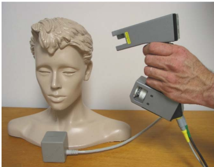
Figure 6: An example of scanning a model. Note the wooden table, placement of the Transmitter, and the position of the Wand.
