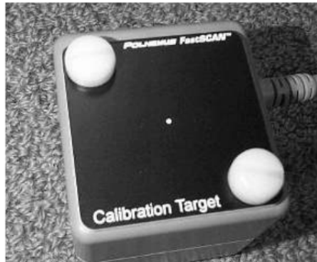
Figure 27: The Transmitter with the Calibration Target attached.
