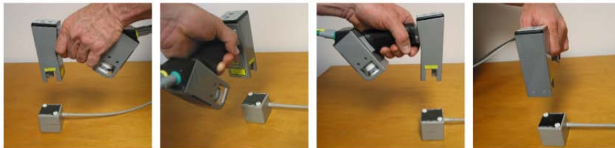
Figure 26: Scanning the Calibration Target at four different angles.
