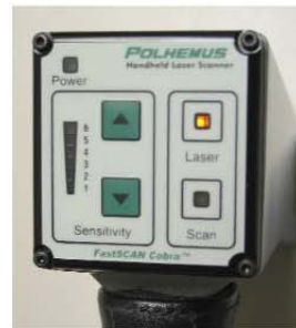
(d) Wand control panel showing Laser-On indicator light (top-right LED)
