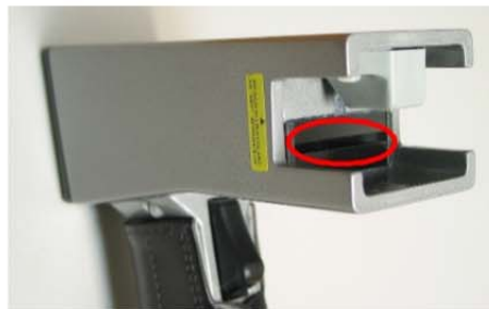
(c) Close-up of the laser aperture (circled), and two-position trigger switch (bottom).
