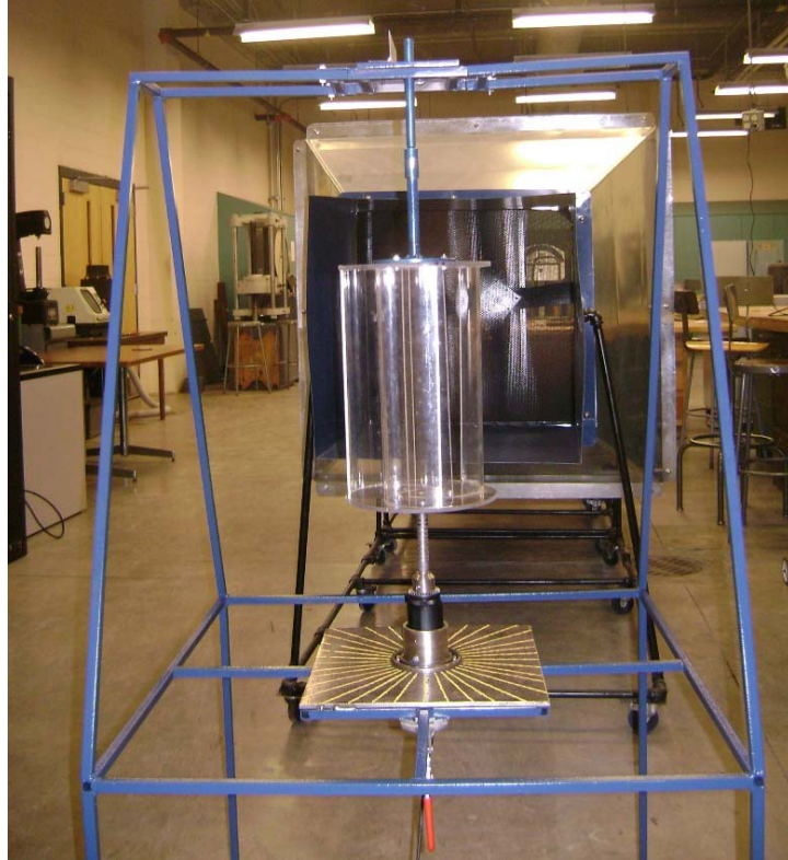
Figure 3.8: Experimental setup of wind tunnel and Savonius rotor model for static torque measurement.
