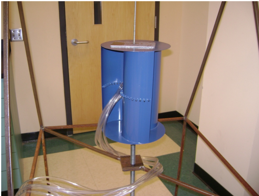
Figure 3.7: A three bladed Savonius rotor Model for pressure measurement.
