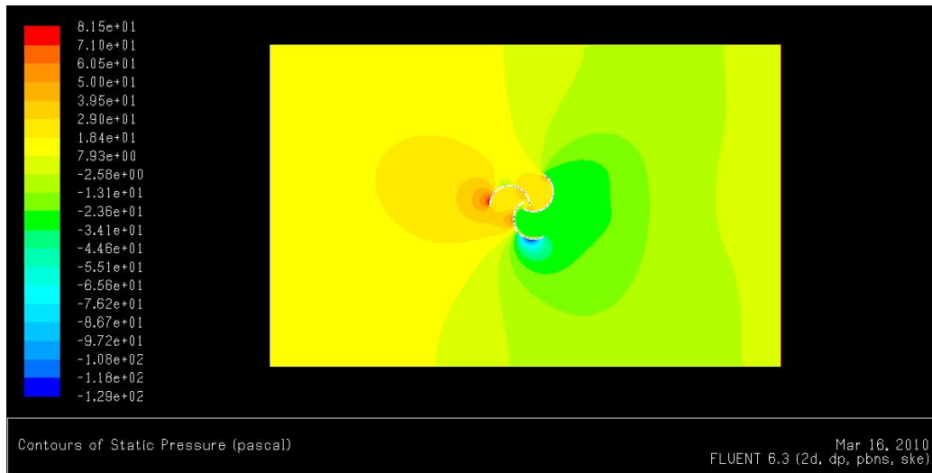
Figure 4.20: Pressure Contour around Savonius rotor Model 2 at Re = 1.19 \times 10^5 .
